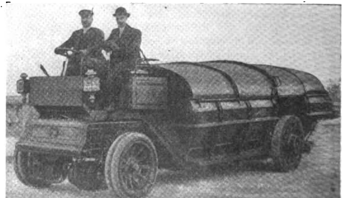
F.R.A.M. 4-ton garbage cart with steel body used in Paris. These trucks weigh about 9 tons and have a speed of 8 miles per hour. The chassis are De Dion-Bouton-Fram products. Batteries are lead and weigh 1 ton each
